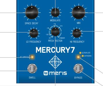
**Pitch Vector:** Sets intra tank pitch interval to: Octave down, slight pitch up, slight pitch down, 5th up, or octave up. Decay, Pitch Vector Mix & Hi/Lo Freq controls all interact to sculpt the intra-tank pitch regeneration **Alt Function: Attack Time** Sets the attack time for the swell envelope
