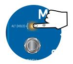
HOLD (L) LED switch on power up (power up takes 3 secs); all of the front panels LEDs will blink 3 times
