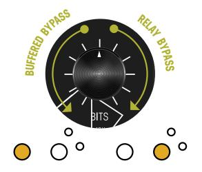
**(L)** LED indicates BUFFERED BYPASS
