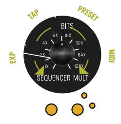
LEDs on front panel blink to indicate EXP, TAP, PRESET. & MIDI
