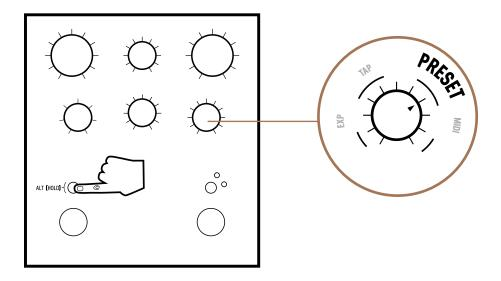
Now with the pedal configuration complete, connect your 4 button switch to the expression pedal input of your pedal using the included TRS cable, and power your Meris pedal normally. You are ready to go.
