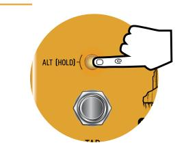
HOLD **(L)** LED switch on power up (power up takes 3 secs); all of the front panels LEDs will blink 3 times
