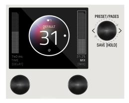
In the <u>EDIT PAGE</u>, if a parameter was assigned as a FAVORITE PARAMETER, a filled in L or R dot will appear to remind which side it was assigned.
