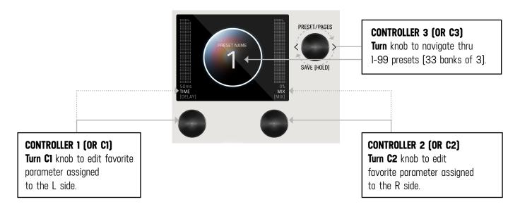
**NOTE:** GRAPHIC VIEW is designed to focus on 1 block and/or 1 parameter at a time per preset. (You have the option to switch to "<u>TEXT VIEW</u>" in GLOBALS -> EDIT PAGE. Favorite Parameters are also available in <u>TEXT VIEW</u>.
